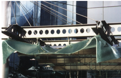
Figure 5: Conventional failure mechanism of tempered laminated
