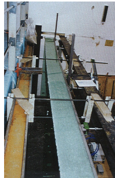
Figure 6: Load test of horizontal glass beam element, all glass sheets broken
